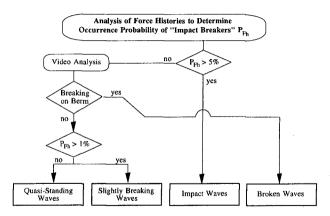
Figure 7. Flow Chart for Identification of Breaker Types for Random Wave Tests
