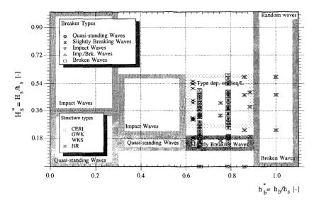
Figure 10.  $H_8^*$  vs  $h_b^*$  for Random Wave Tests (All Data Sets)
