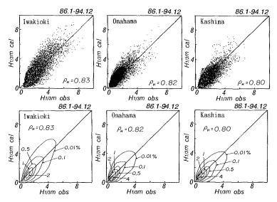
Figure 4. Scatter Diagram between Hindcast and Measurement for Significant Waves and Contour Plot of Relative Occurrence Frequency in a Segment of Wave Height at 3 Stations
