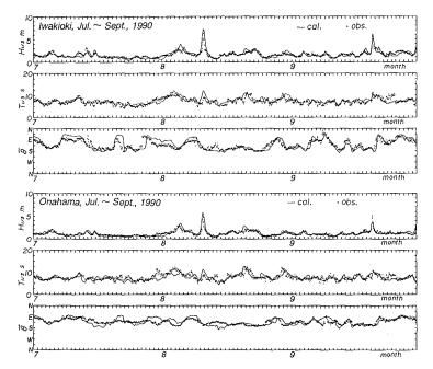
Figure 3. Comparison between Hindcast and Measurement for Time Variations of Significant Waves and Mean Wave Direction over 3 Months.
