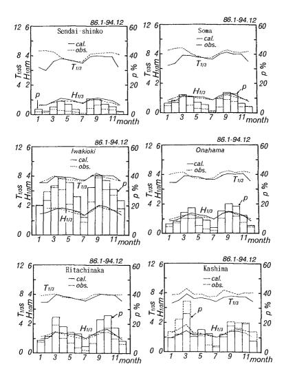
Figure 5. Comparison of Hindcast and Measurement for Monthly Variations of Mean Significant Waves and Occurrence Rate of High Waves
