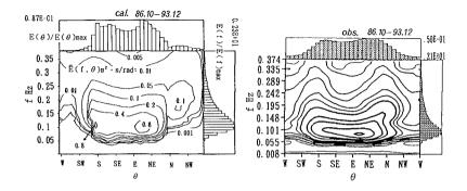
Figure 10. Comparison of Hindcast and Measurement for Directional Spectrum, Directional Energy and Frequency Spectrum Averaged over 7 Years
