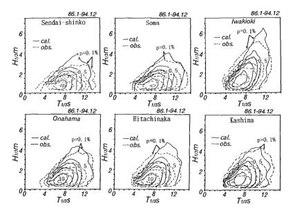
Figure 7. Comparison of Hindcast and Measurement for Correlation between Wave Height and Wave Period
