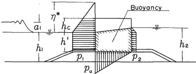
Figure 7. Tsunami Wave Pressure Distribution
