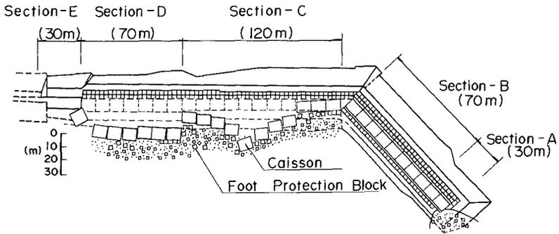
Figure 3. Caisson Sliding at the North Breakwater
