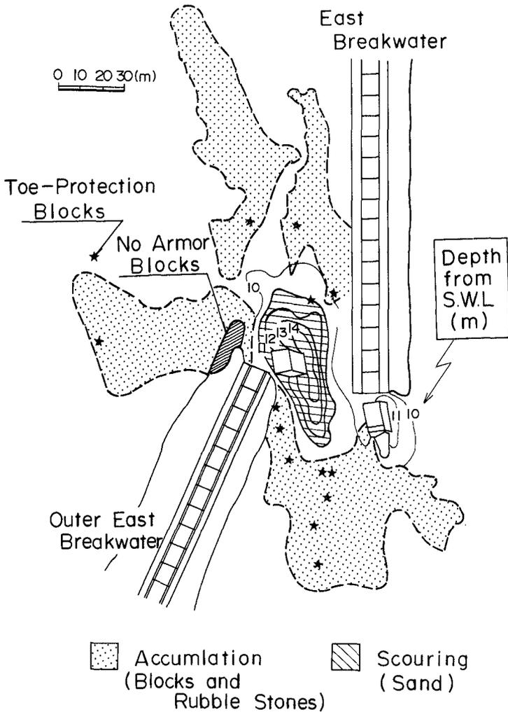
Figure 5. Scouring at the Narrow Opening
