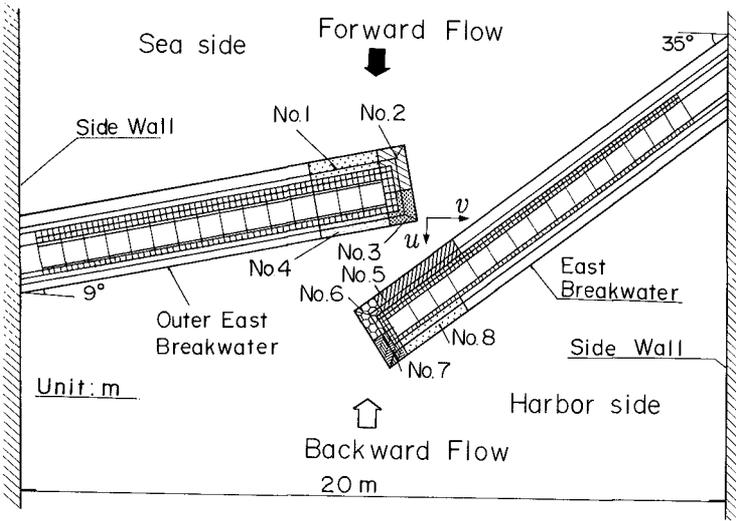
Figure 9. Breakwater Model in the 3-D Basin
