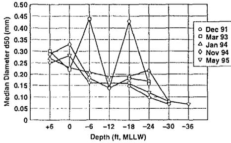
Figure 5. Cross-shore Comparison of  $d_{50}$  Median Diameter, Line 19
