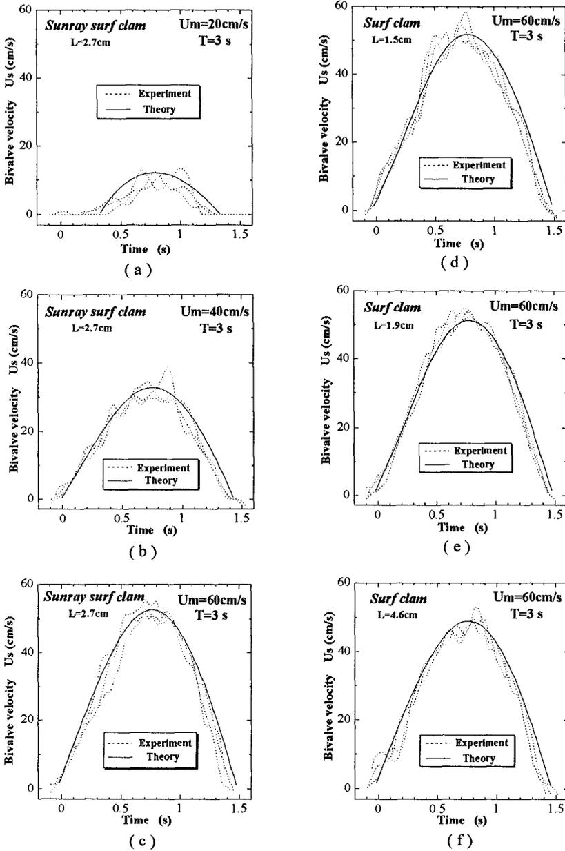
Fig.7 Moving velocity of the bivalves on a smooth surface fixed bed
