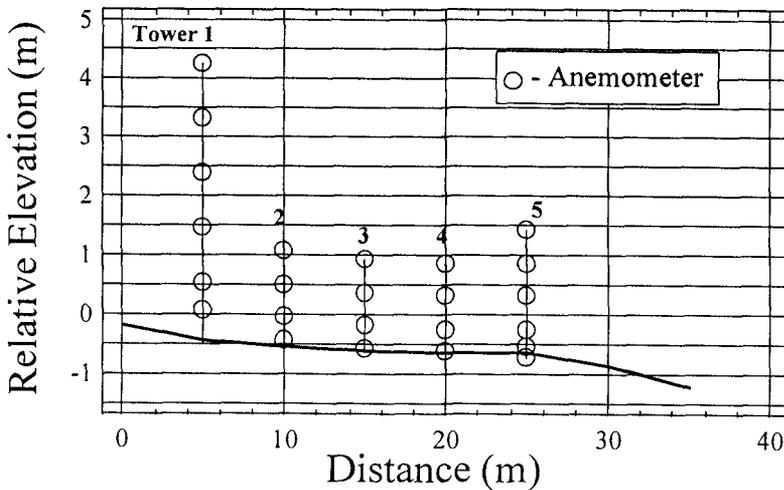
Figure 2: Instrument configuration on January 13, 1993.
