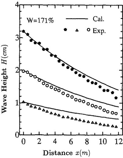
Fig. 8 Comparison between calculated and measured wave damping.
