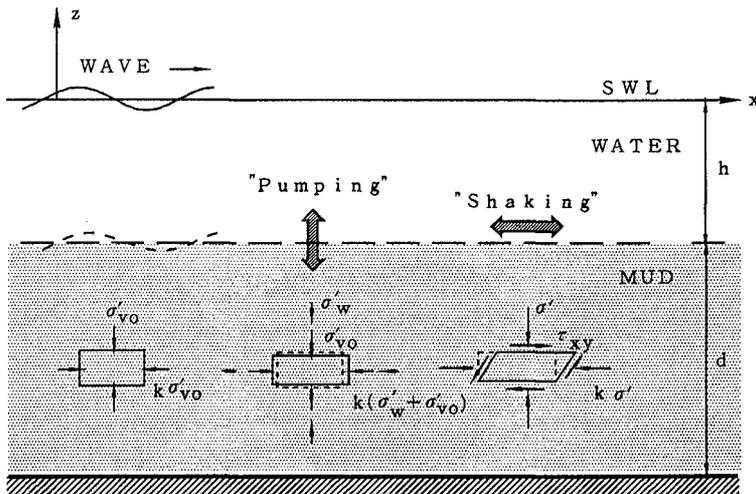
Fig. 6 Idealized stress state in mud bed under waves.
