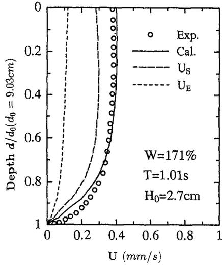
Fig. 9 Calculated and measured mud mass transport velocity.
