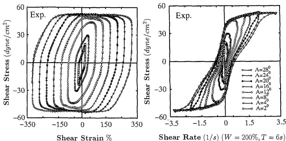
Fig. 1 (a) Shear stress vs. shear strain (effects of the angular amplitude).
