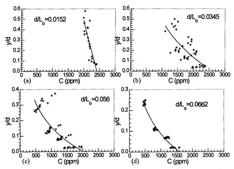
Figure 7 The vertical concentration distribution for the different relative water depth
