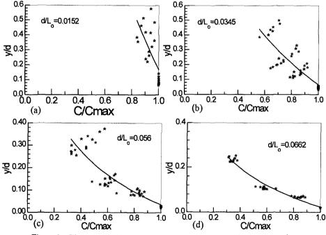
Figure 8 The vertical distribution of dimensionless suspended concentration
