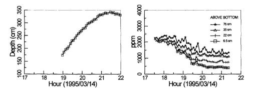
Figure 6 Time series of the water level and its corresponding suspended concentration
