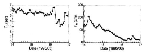
Figure 3 Time series of wave period and wave height at -20m water depth
