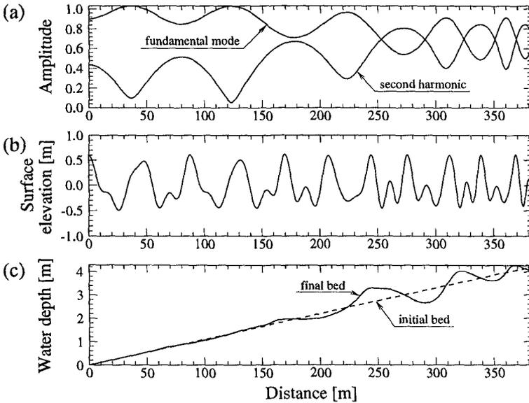
Figure 6: Prediction of wave and morphology evolution under nonlinear waves without group-like modulation (simulation of an extreme storm event with  $T_p = 6.9$  s): (a) amplitude of the two first harmonic modes, (b) free-surface elevation, (c) initial and final bed.
