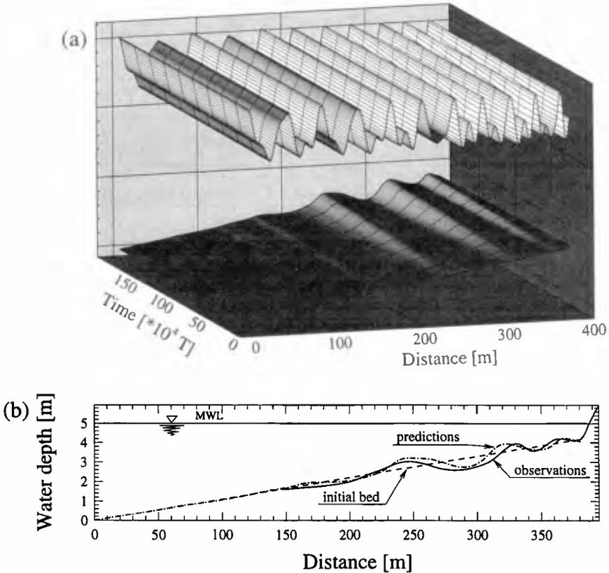
Figure 7: Prediction of morphology evolution under nonlinear waves without group-like modulation (simulation of an extreme storm event with  $T_p = 6.9\text{s}$ ): (a) temporal evolution of waves and morphology, (b) predicted and observed multibar morphology.
