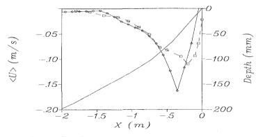
**Figure 3a.** Undertow. Case P. ———— Depth,  $-\Box$  – data points, —— $\diamond$ — Numerical solution.
