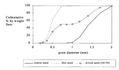
Figure 5. Grading curves.
