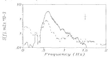
Figure 2. Wave spectra for case P outside the surf zone and close to the shoreline. x=-2m (d=200mm), ---x=-0.05m (d=10mm).
