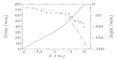
**Figure 1a**. RMS wave height across the surf zone, case P. ——— Depth,  $\Box \Box \Box \Box$  Data points, ——— Numerical solution.
