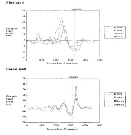
Figure 6. Change in bed elevation from original profile, case K.
