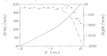
**Figure 1b**. RMS wave height across the surf zone, case K. ——— Depth ,  $\Box \Box \Box \Box$  Data points, — — — Numerical solution.
