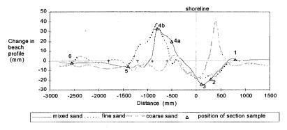
Figure 8b. Change in bed elevation from original profile, case K.
