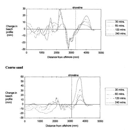
Figure 7. Change in bed elevation from original profile, case P.
