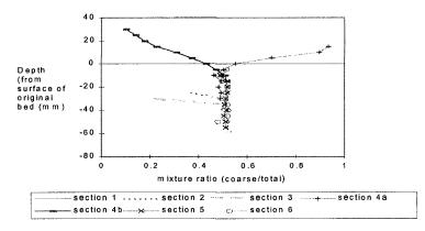
Figure 8c. Variation in mix ratio with depth at six cross-shore locations, case K.
