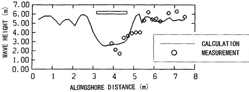
Fig. 5 Alongshore distribution of breaking wave height.
