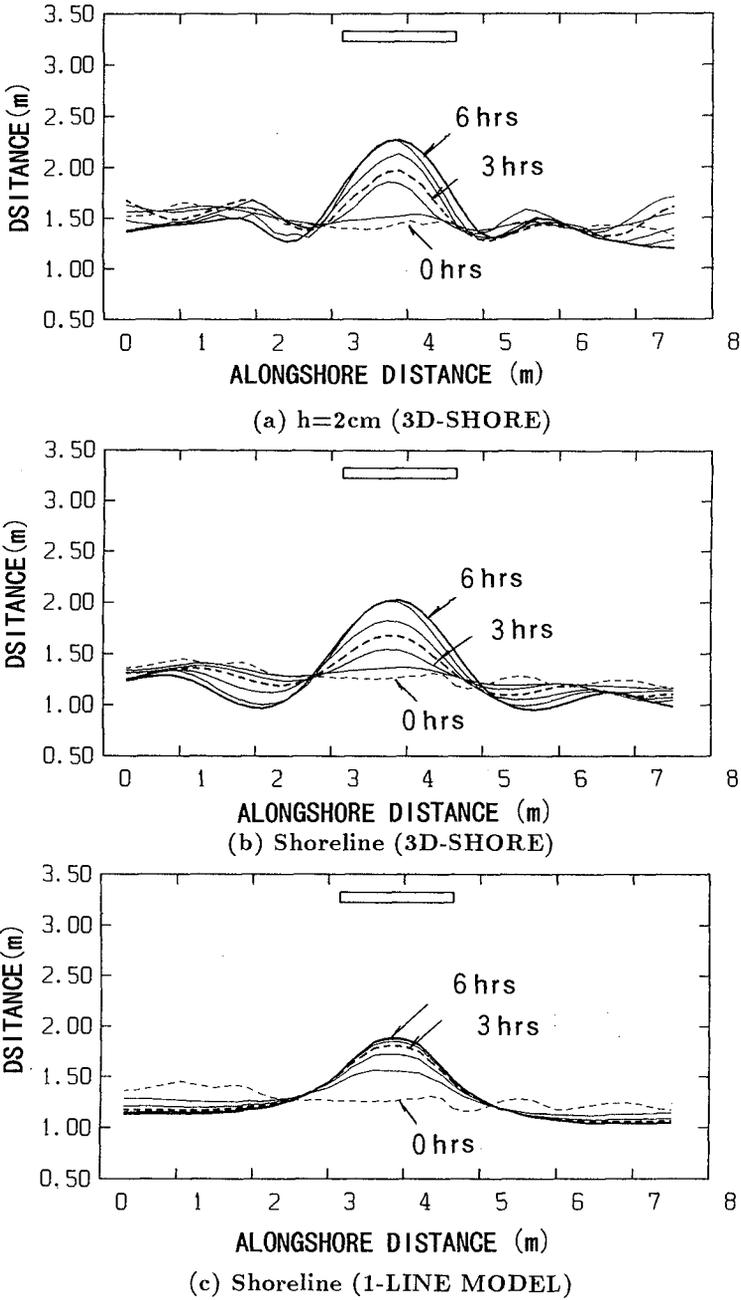
Fig. 8 Time-evolution of the calculated depth contours.
