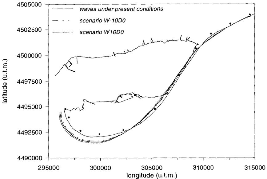
Figure 7. Prediction of the Ebro delta coastline evolution for the year 2050 under present conditions and assuming two scenarios of wave height change (*W10D0*: 10% increase in wave height, *W-10D0*: 10% decrease in wave height).
