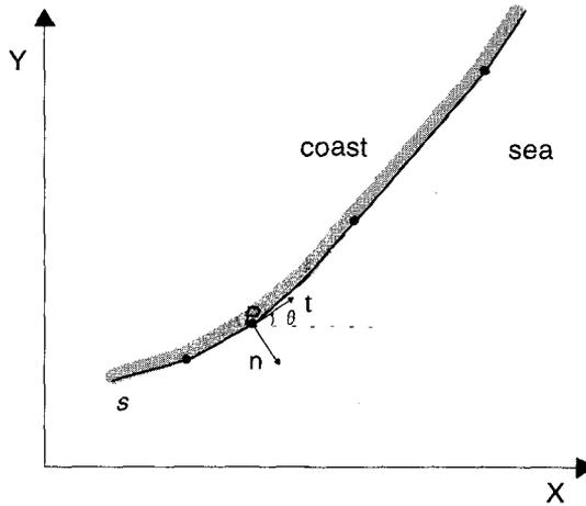
Figure 5. Curvilinear coordinate system.
