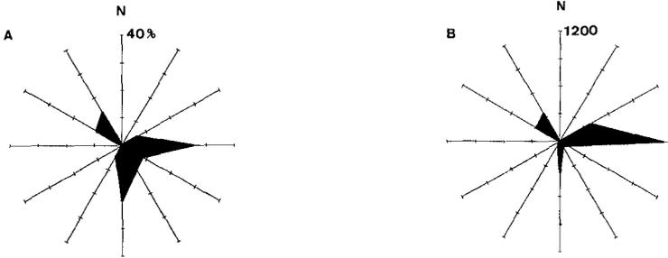
Figure 3. (a) Offshore directional wave distribution. (b) Offshore directional distribution of the yearly-integrated wave energy flux (calculated as  $H_s^2 T_p f$ ) (Jiménez, 1996).
