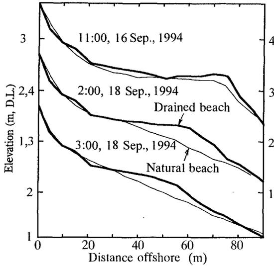
Figure 8 Comparisons of Profiles on the Natural and the Drained Beaches.
