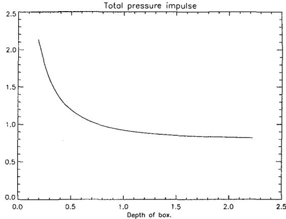
Figure 9: Total impulse on deck against depth  $a$ .
