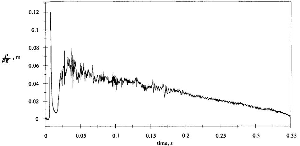
**Figure 5: Typical impact pressure trace at model scale**
