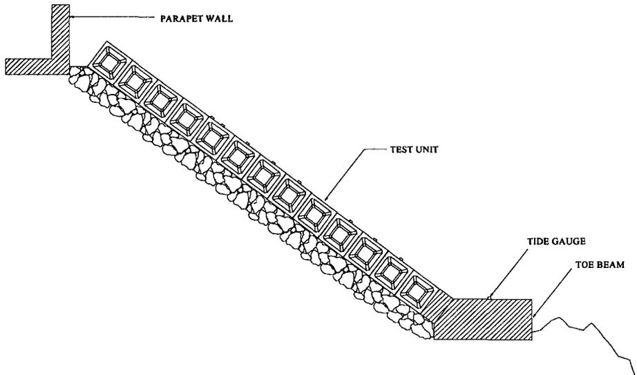
**Figure 1: Typical cross-section of LaCollette Breakwater, Jersey, UK**
