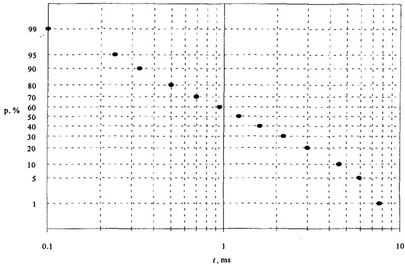
**Figure 6: Log-normal distribution of impact pressure rise times, model**
