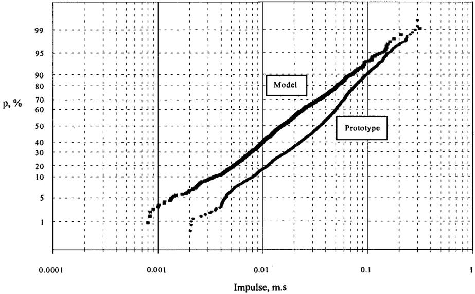
Figure 7: Comparison of impact impulses using Froudian scaling
