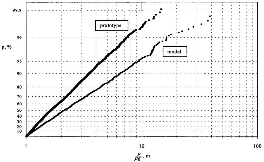
Figure 8: Comparison of pressure magnitudes using Froudian scaling
