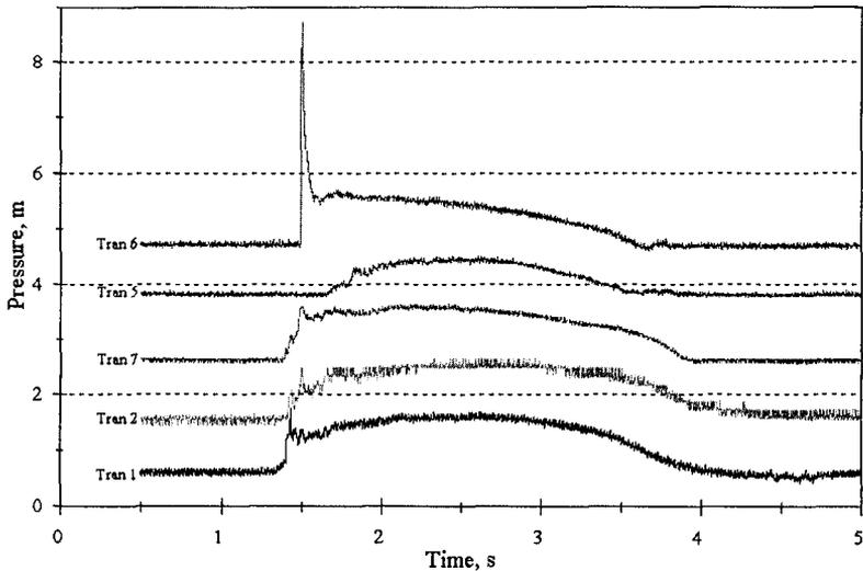
**Figure 2: Typical pressure traces measured at prototype scale**
