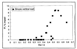
Figure 6 Influence of H<sub>st</sub>/d on P<sub>1%</sub> for simple walls
