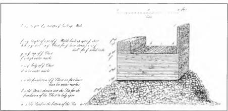
Figure 2 Timber caisson used for the Greate Mole at Tangier, 1677
