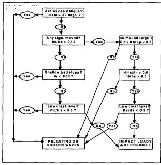
Figure 3 Impact breaking conditions, derived from Goda (1985)
