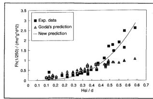
Figure 7 Dimensionless force against H<sub>sl</sub>/d for simple walls
