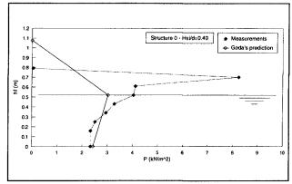
Figure 11 Vertical distribution of pressures, H<sub>s</sub>/d=0.4, simple wall
