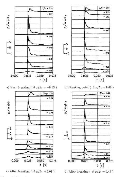
Figure 3: Time histories of the plunging wave pressure recorded on the wall at different locations.
