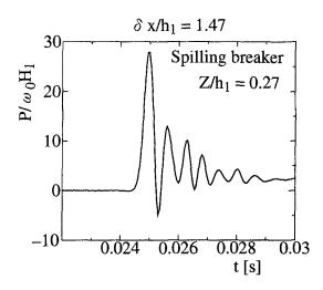
Figure 5: Oscillations in the time history of the spilling wave pressure.
