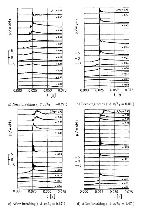
Figure 4: Time histories of the spilling wave pressure recorded on the wall at different locations.
