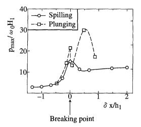
Figure 8: Variation of the peak value in the vertical distribution of maximum pressure with wall locations.
