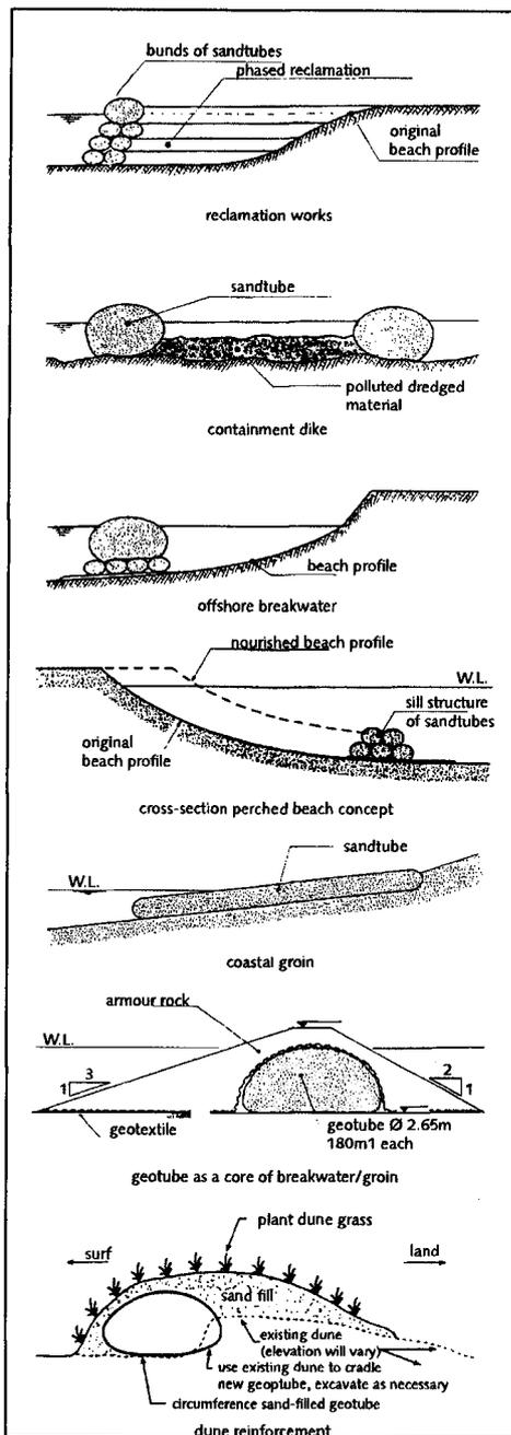
Figure 2. Coastal applications of geotubes/containers
