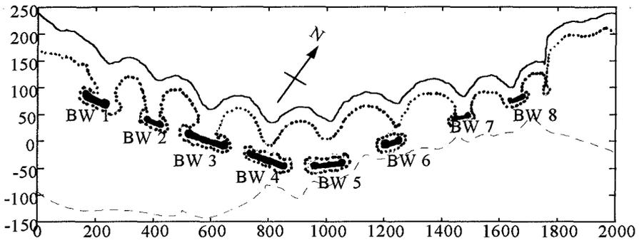
**Figure 3.** Elmer frontage, showing numbering scheme for breakwaters, and levels of highest (solid line) spring, mid (dotted line) and lowest spring (dashed line) tides
