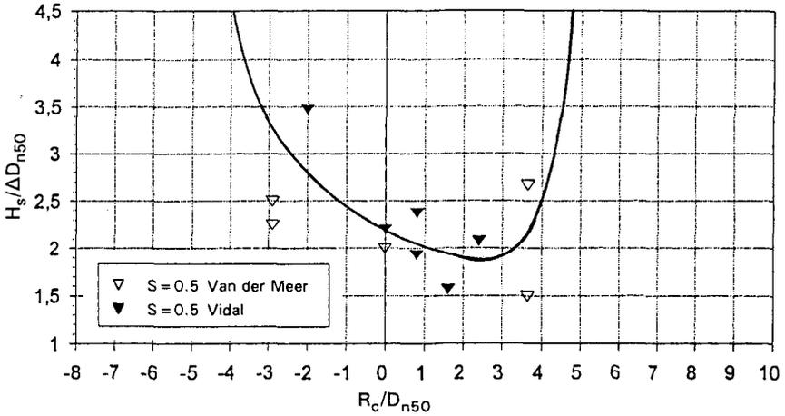
Figure 5. Stability rear for start of damage
