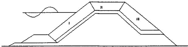
Figure 1. Division of armour layer in three segments
