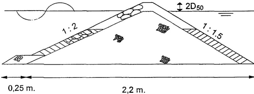
Figure 11. Tested cross-section
