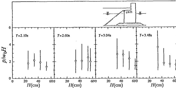
Fig. 13 Impulsive pressure intensity on a joint plate.
