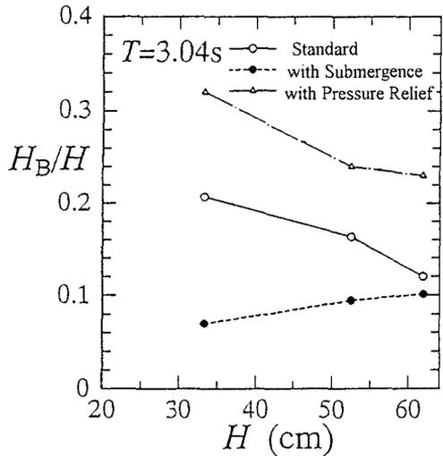
Fig. 8 Water level oscillations in backfill region.
