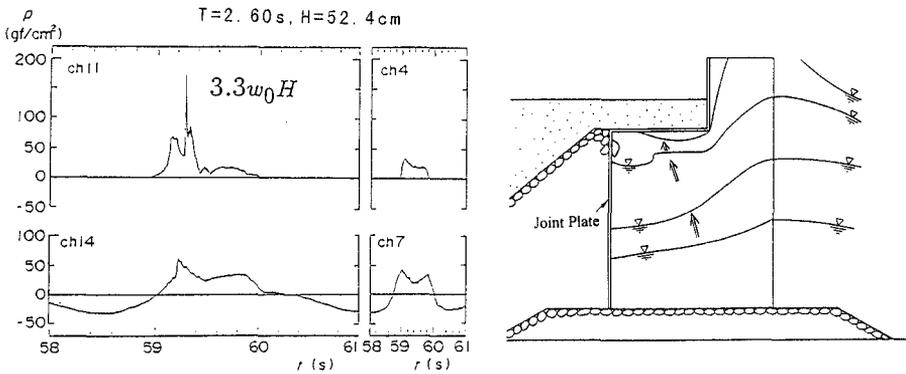
Fig. 12 Generation of impulsive pressure on joint plates.
