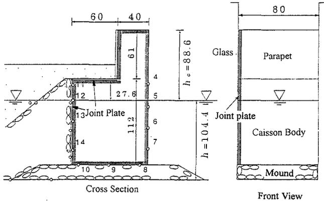
Fig. 11 Seawall model with a caisson joint plate.
