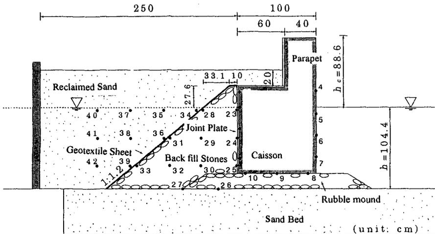
Fig. 3 Cross section of the standard seawall model.
