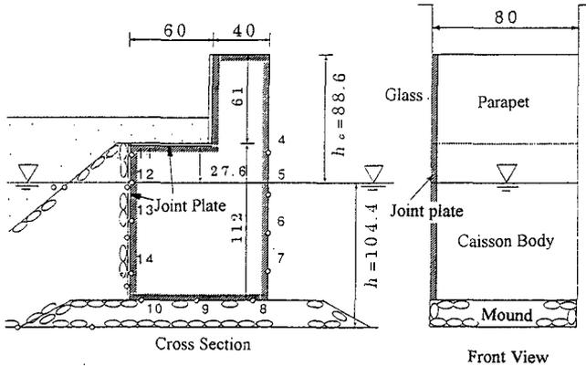
Fig. 11 Seawall model with a caisson joint plate.
