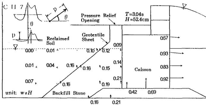
Fig. 7 Distribution of positive peak pressure using pressure relief opening.
