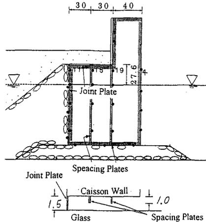
Fig. 14 Spacer plates to reduce the impulsive pressure.
