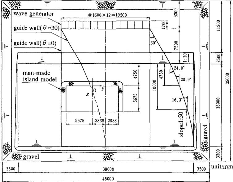
Fig.2 Multidirectional wave basin and man-made island model
