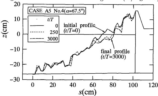
Fig.11 Profiles deformed with functional check wave( $H/H_D=1.24$ )
