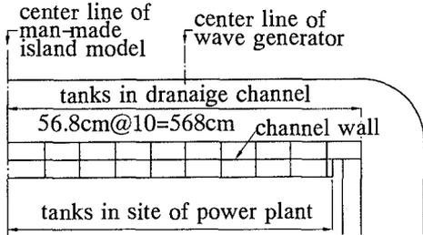
Fig.3 tanks to measured overtopping volume
