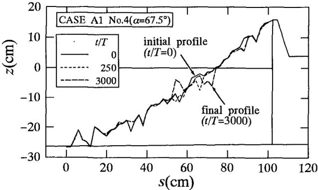
Fig.10 Profiles deformed with design wave( $H/H_D=1.0$ )
