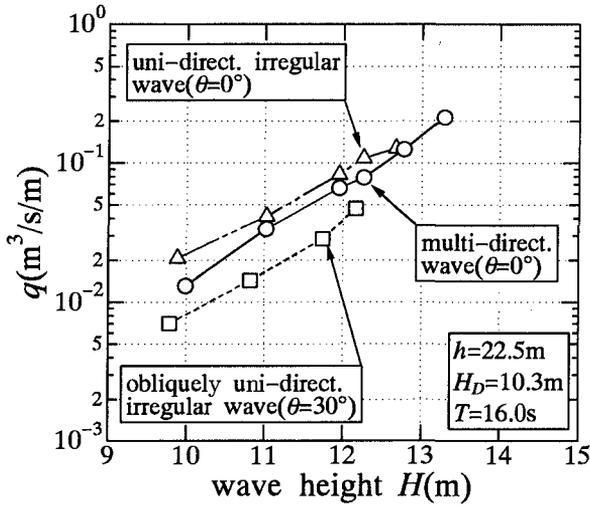
Fig.9 Overtopping rate  $q$  dependent on wave directionality
