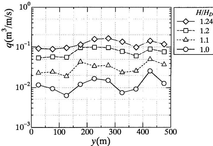
Fig.6 Local overtopping rate along seawall due to multidirectional wave
