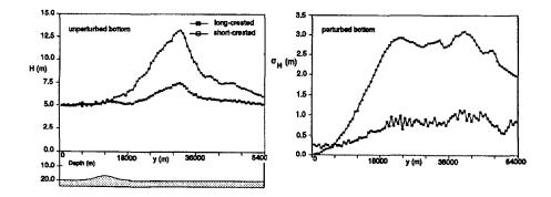
Figure 4: Results obtained by the HISWA model (Holthuijsen and Booij, 1994.) for the circular shoal. a). Wave heights along centerline profile for circular shoal with unperturbed bottom; b). The standard deviations of the wave height for the perturbed bottom.
