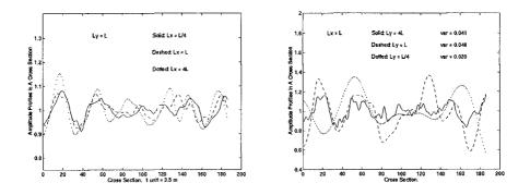
Figure 11: Cross-section amplitude profiles obtained by the REF/DIF model, nonlinear version. L: water wave length,  $L_x$  and  $L_y$ : water depth correlation lengths in wave propagation and transverse directions, respectively. Wave period = 5 sec, Mean water depth = 5 m. Standard deviation of water depth = 0.5 m. Distance from where waves start: 700 m.
