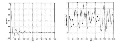
Figure 1: A sampled correlation function and a generated water depth variations for 2-D case. a). Correlation function; b). Water depth variation. The correlation length is about 30 grid sizes.
