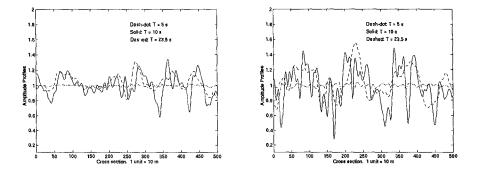
Figure 12: Cross-section amplitude profiles obtained by the REF/DIF model, nonlinear version, for incident waves of different wave periods T. Bathymetry in Duck, NC is applied. Distance from the incident waves, left figure: 1 km; right figure: 2 km.
