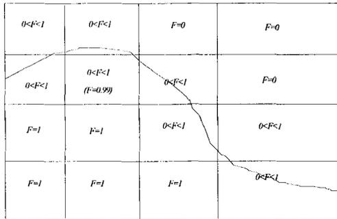
Figure 1. Illustration on the type of fluid and void cells considered by the VOF wave model.
