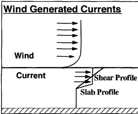
Figure 7. Wind generated current profiles for design use.
