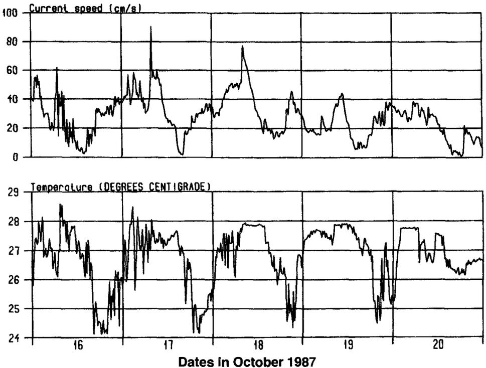
Figure 8. Current and temperature measured by Aandera current meter at -50 meter.
