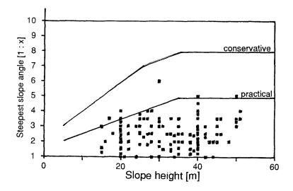
Figure 3 Actual flow slides compared to model results: Slope angle of steepest part of the slope as a function of slope height
