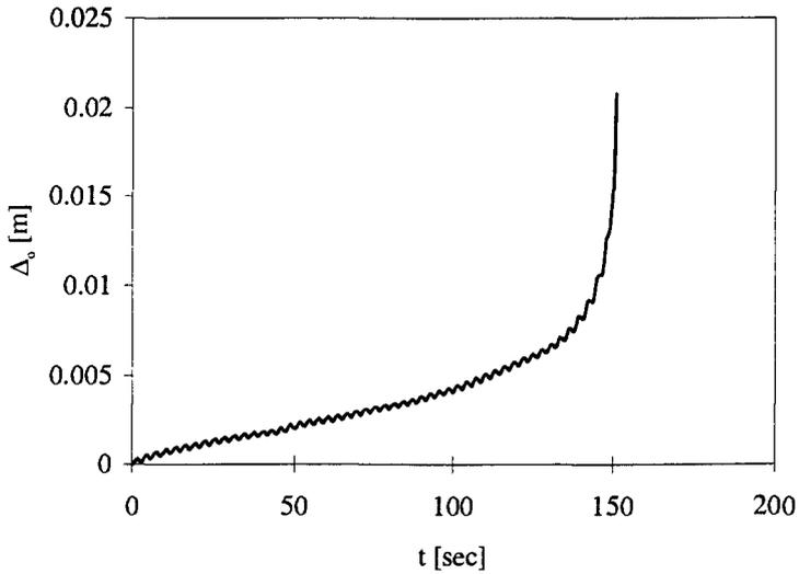
Figure 2. Measured vertical displacement history in Experiment F4.
