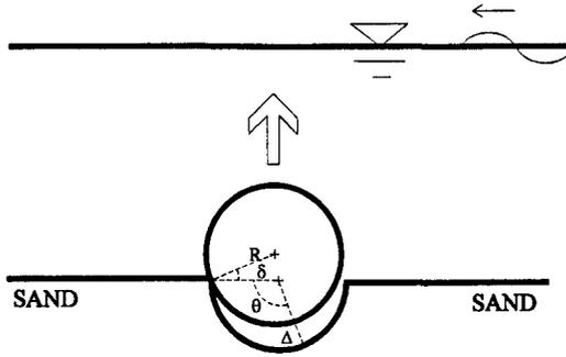
Figure 1. Configuration of the breakout of a half-buried pipe from sea bed due to wave action.
