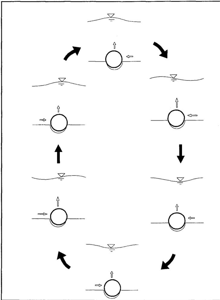
Figure 3. Movement of the pipe during one wave cycle.
