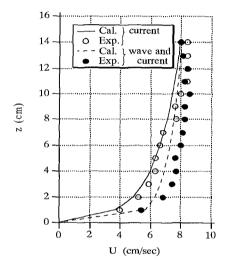
Fig. 4 Vertical distribution of mean current velocity in the case of wave and current coexisting field. (h=20cm, D=0.012cm, current ,U=7.0cm/sec ; wave and current :T=1.5sec, H=6cm, U=7.5cm/sec )
