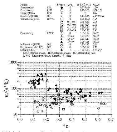
Fig. 5 Relation between non-dimensional diffusion coefficient and grain roughness Shields' number
