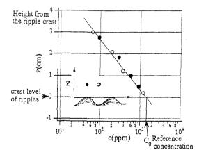
Fig. 3 Examples of vertical distributions of time averaged suspended sediment concentration measured at the crest and the trough of the ripple. (h=20cm, D=0.012cm, T=1.5sec, H=6cm)
