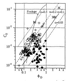
Fig. 8. Relation between measured reference concentration  $C_0$  and grain roughness Shields' parameter  $\phi_D$ .
