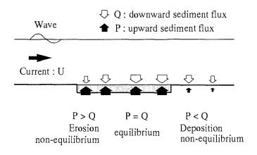
Fig. 1 Typical example of non-equilibrium suspended sediment transport
