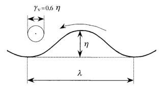
Fig. 7 Vortex generated on the ripple
