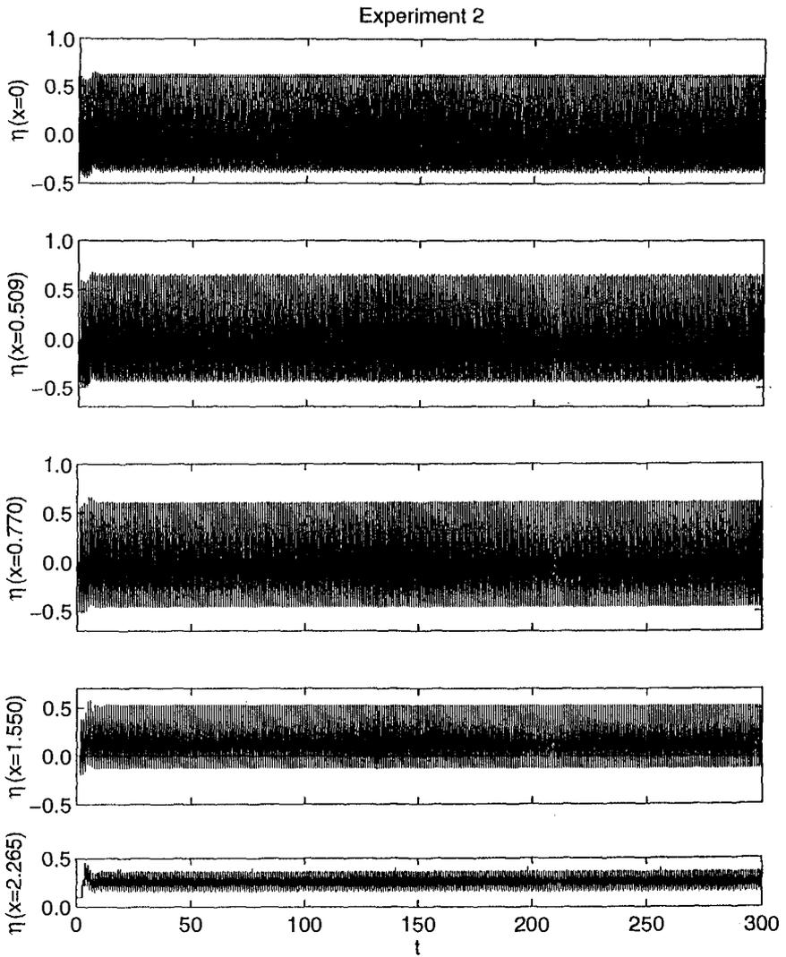
Figure 2: Computed Temporal Variations of Free Surface Elevation  $\eta$  at  $x = 0, 0.509, 0.770, 1.550$  and  $2.265$ .
