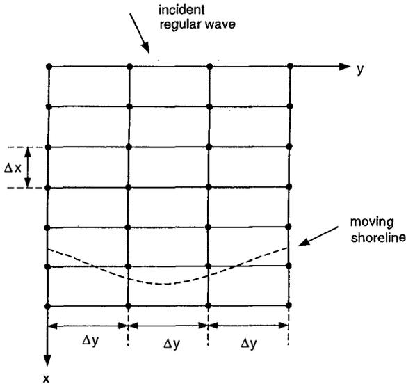
Figure 1: Finite Difference Grid for Numerical Model
