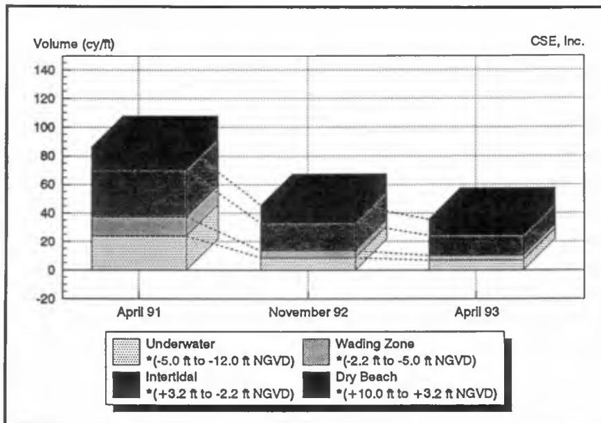
**FIGURE 5.** Average unit-volume beach change since nourishment (February 1991) as a function of contour interval\* within the Hunting Island project area (stations 3+42 to 83+31). Note: Higher loss rate for lower beach lenses is thought to be related to variations in grain size along the profile. After Kana and Andrassy (1993).
