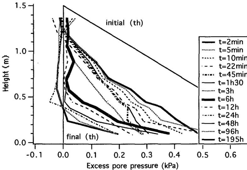
Fig.4: Evolution of excess pore pressure profiles with time
