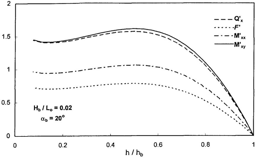
Figure 3 - Evolution of dimensionless volume, energy, and momentum flux components, defined in Eq.(9), for a breaker angle of  $20^\circ$ .
