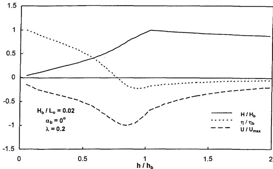
Figure 5 - Dimensionless wave height, set-up, and cross-shore current generated by numerical solution to Eqs. (1), (4), (5), and (6), for a breaker angle of  $0^\circ$ .
