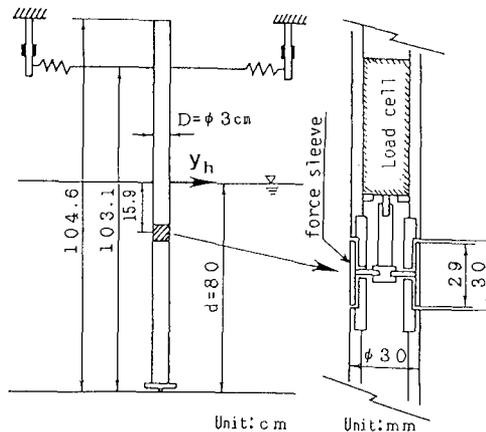
Fig. 2 Experimental Set-up (Force Sleeve and Load Cell)
