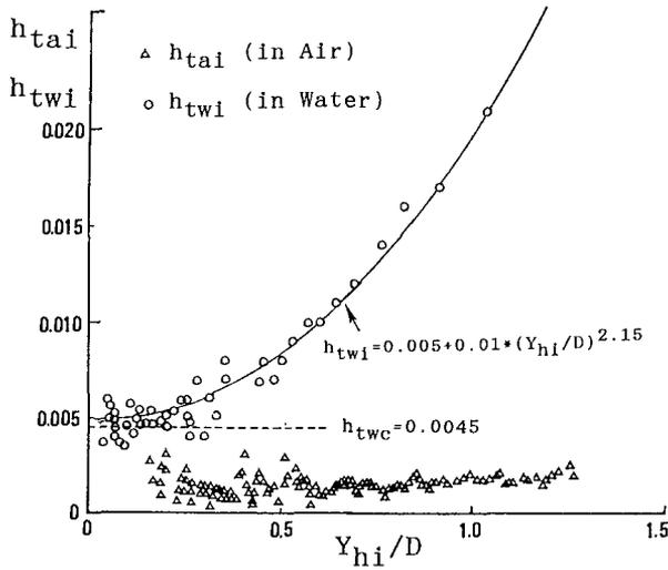
Fig. 5 Variation of Damping Factor with  $Y_{hi}/D$
