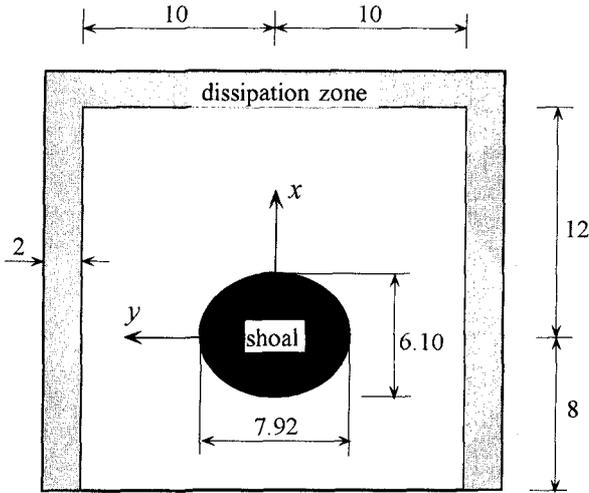
Fig. 3: The computational domain (all numbers are measured in meters)
