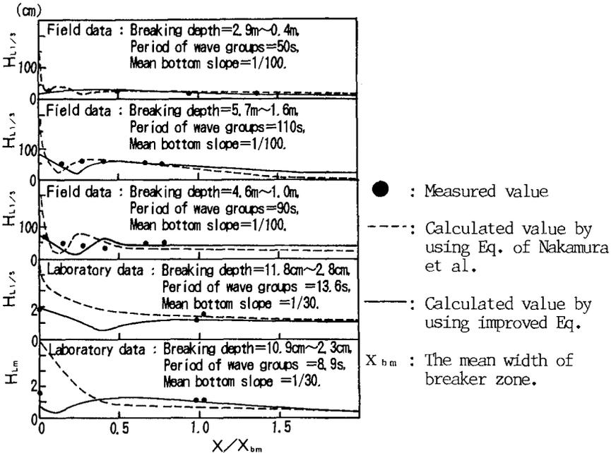
Fig.4 Comparison between observed data and predicted curve.
