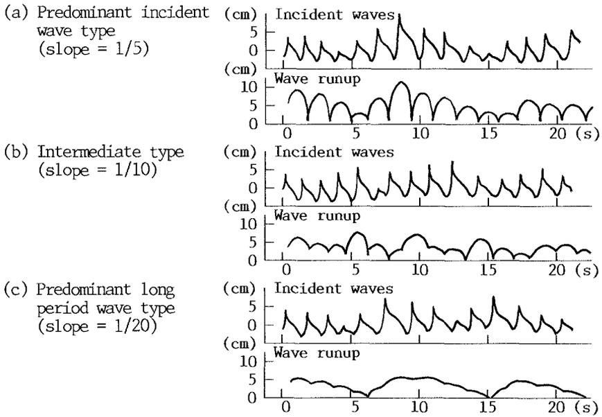
Fig.1 Type of wave run-up profiles.
