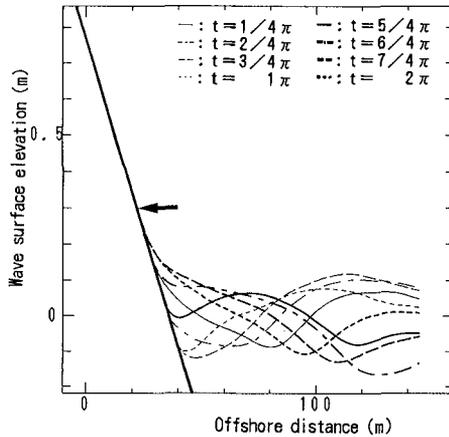
Fig.10 An example of long period wave runup. (The arrow shows  $R_{Lm}$  calculated by Eq.(10))
