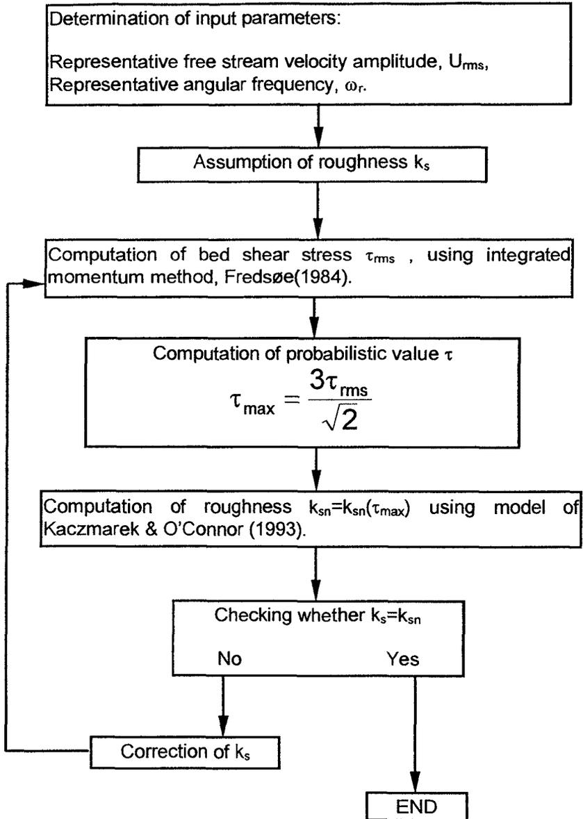
Figure 6: Modified iteration scheme for spectral waves.
