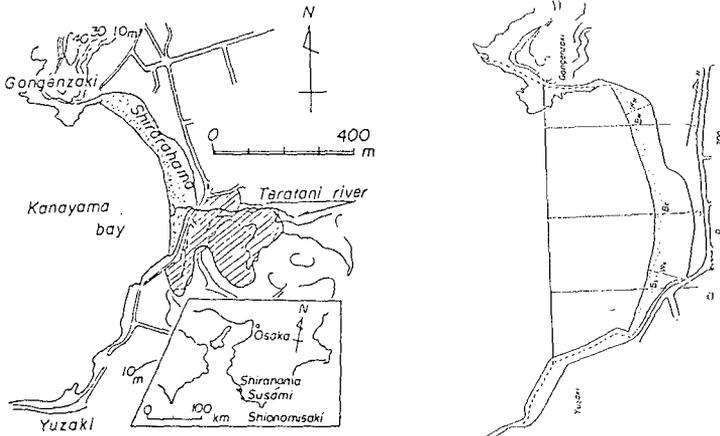
(a) Location and sediment source area (b) Survey lines of beach width
