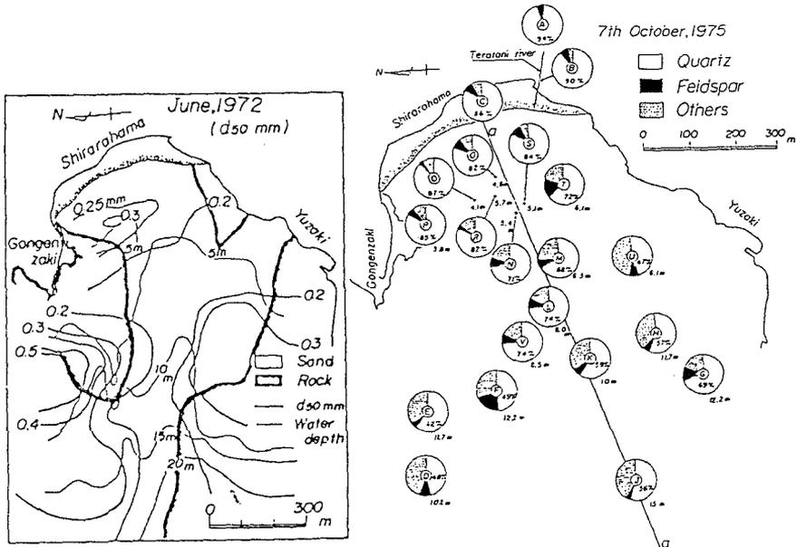
(a) Median diameter of sediment (b) Mineral composition of sediment
