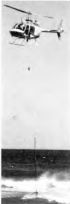
Figure 8. Survey stand deployment
