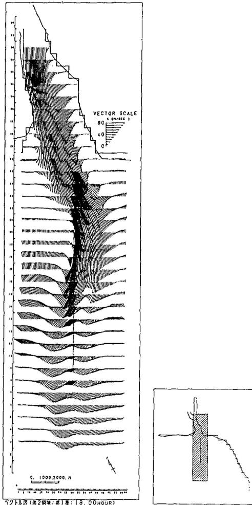
**Fig.4** Current Vector Distribution (at 18:00, 1st layer)
