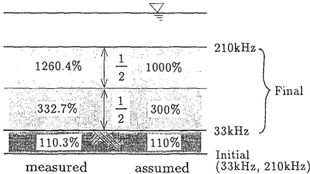
Fig.6 Measured and Assumed Water Content of Mud
