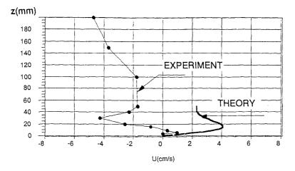
Fig.-7 Vertical Distribution of Mean Currrent
