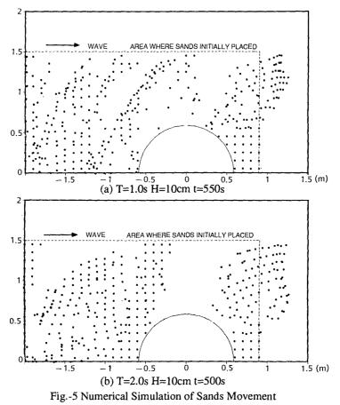
included in the simulation. Important findings are the sand particles disappear at the side of the cylinder both in the simulation and the experiment. In other hand, the side of the cylinder is always accretion area in the bathymetric change experiment (see fig.-1(a) and (b)).
