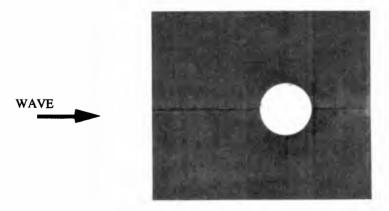
(b) T=2.0s H=10cm t=1 min. Photo-1 Movement of Polyethylene Beads around a Large Circular Cylinder
