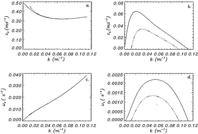
Figure 1: Linear stability for the TG86 model. (a) Real phase velocity, (b) imaginary part of phase velocity, (c) radial frequency, and (d) growth rate. Solid line:  $c_d = 0$ . Chained line:  $c_d = .003$ . ( $c_f = .009$ ).
