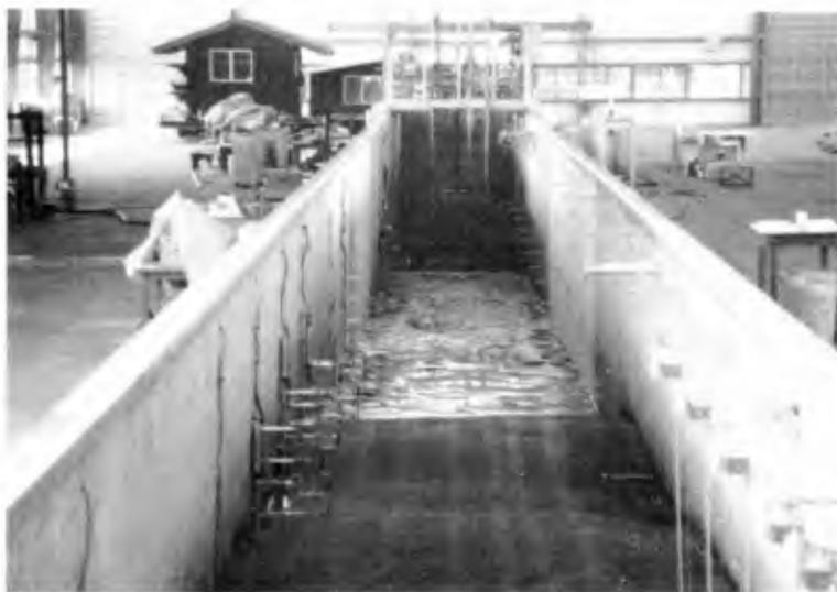
Fig. 2. Close-up view of LWT with SUPERTANK instrumentation
