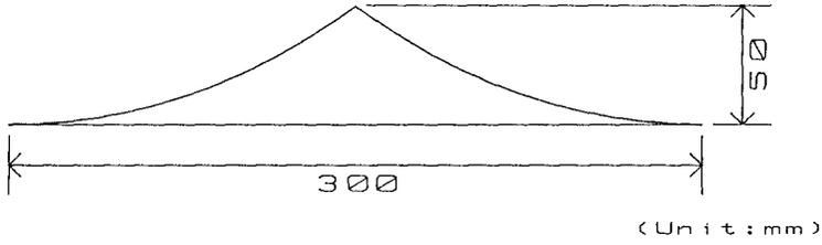
Fig.1 Fixed ripple model with a sharp crest.
