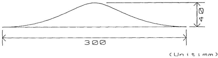
Fig.3 Fixed ripple model with a round crest.
