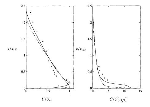
Figure 3: Predicted mean flow profiles for saline gravity current. Symbols represent laboratory experiments by Ellison and Turner (1959). Line types as in Figure 2. The slope is  $\beta = 0.24$  radians.
