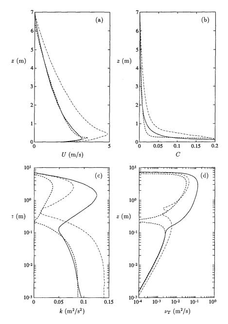
Figure 2: Predicted profiles for self-accelerating turbidity current. Full line; Reynolds stress model, dashed line;  $(k-\varepsilon)$  model, dashed-dotted line;  $(k-\varepsilon)$  model with bridge across the k profile dip.
