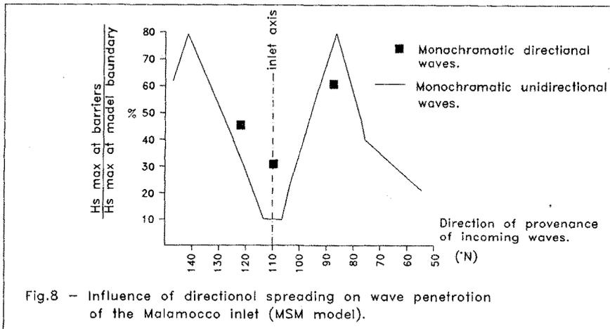
Fig.8 - Influence of directional spreading on wave penetration of the Malamocco inlet (MSM model).
