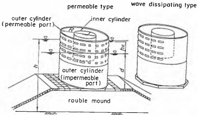
Fig. 1 Conceptual Figure of Dual Cylindrical Caisson
