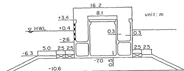
Fig. 6 Cross Section of Sliding Test Caisson
