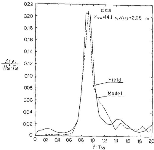
Fig. 10 Wave Spectra in the Field and Laboratory
