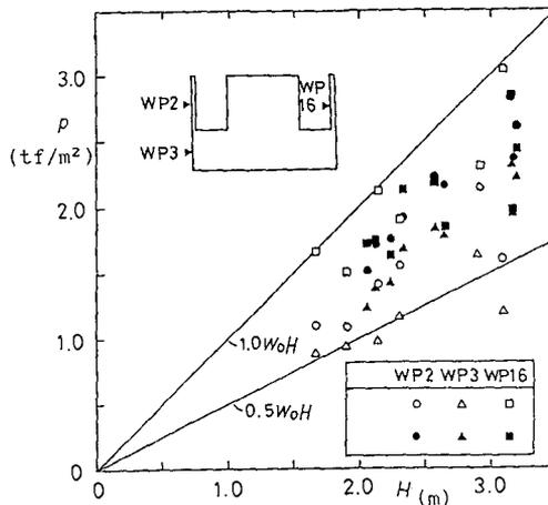
Fig. 9 Pressure Intensities in the Field Experiments
