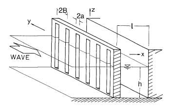
Figure 1. Slit-type breakwater.
