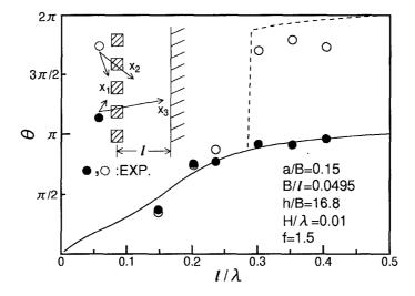
Figure 5. Comaparison between theoretical and experimental data for phase differences between inside and outside the chamber,  $x_1/l = -0.125$ ,  $x_2/l = 0.125$ ,  $x_3/l = 0.917$ .
