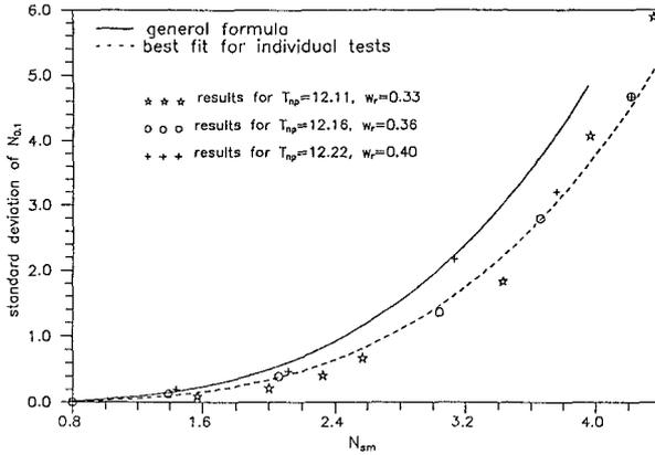
Figure 6. Comparison individual test variations with Equation 6
