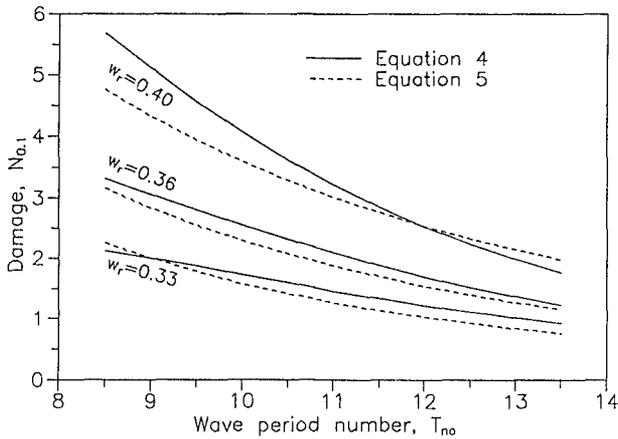
Figure 3. Comparison of the two equations for  $N_{sm} = 2,75$
