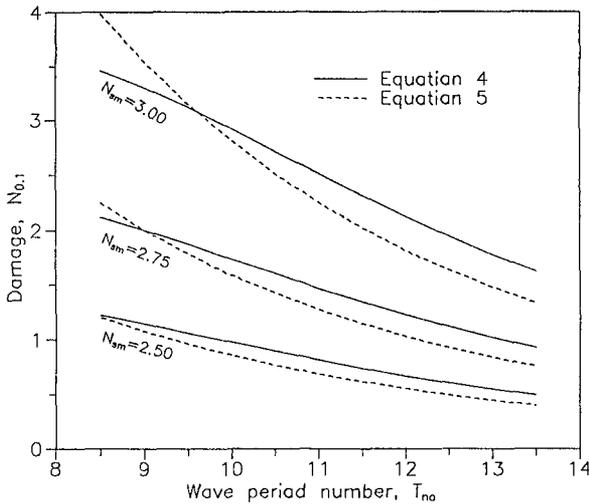
Figure 4. Comparison of the two equations for  $w_r = 0,33$
