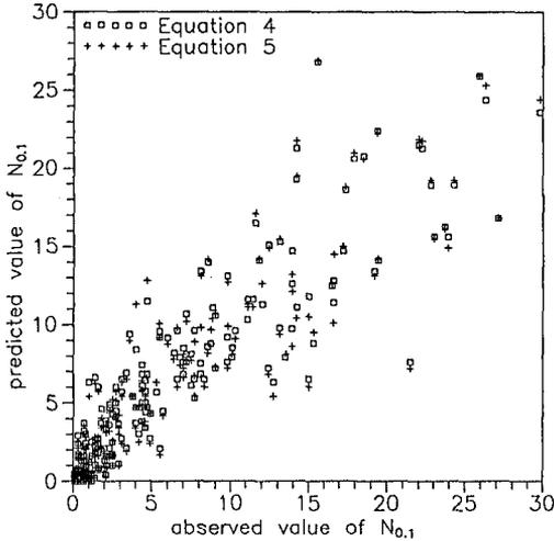
Figure 2. Predicted versus observed dolos stability
