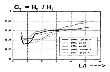
Figure 7: Performance of the breakwater
