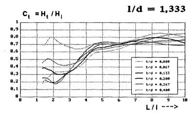
Figure 2: Wave height reduction at the plate [Dauer, 1984]
