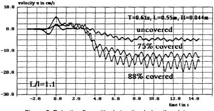
Figure 6: Pulsating flow with obstruction below the plate
