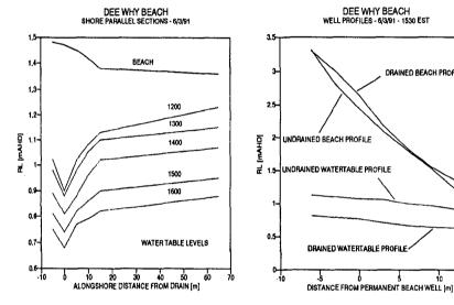
Figure 5 — Effects of a single drain on the watertable at various times (EST)
