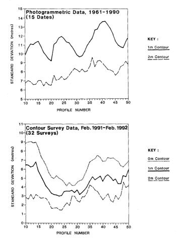
Figure 8 — Contour excursion standard deviation for photogrammetric data and survey data
