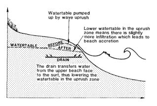
Figure 1 — Effect of the strip drain on the watertable
